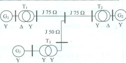
c) For the shown network, construct the admittance matrix. It is required to reduce the network size by eliminating buses 3 and 4. Derive the reduced admittance matrix and draw the network after reduction. (15)
